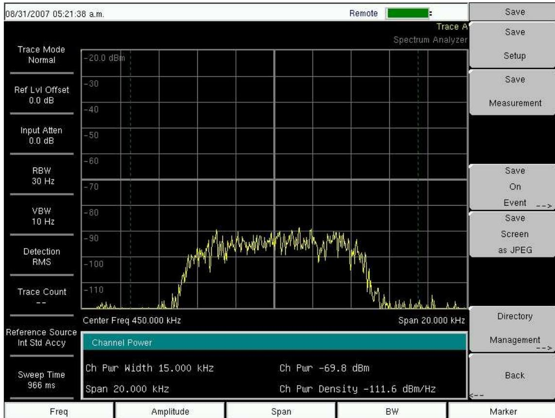
**Figure 2 ID-800 450 kHz IF Prior to Detection (Blue Dot in Figure 1) with No Signal Applied**
