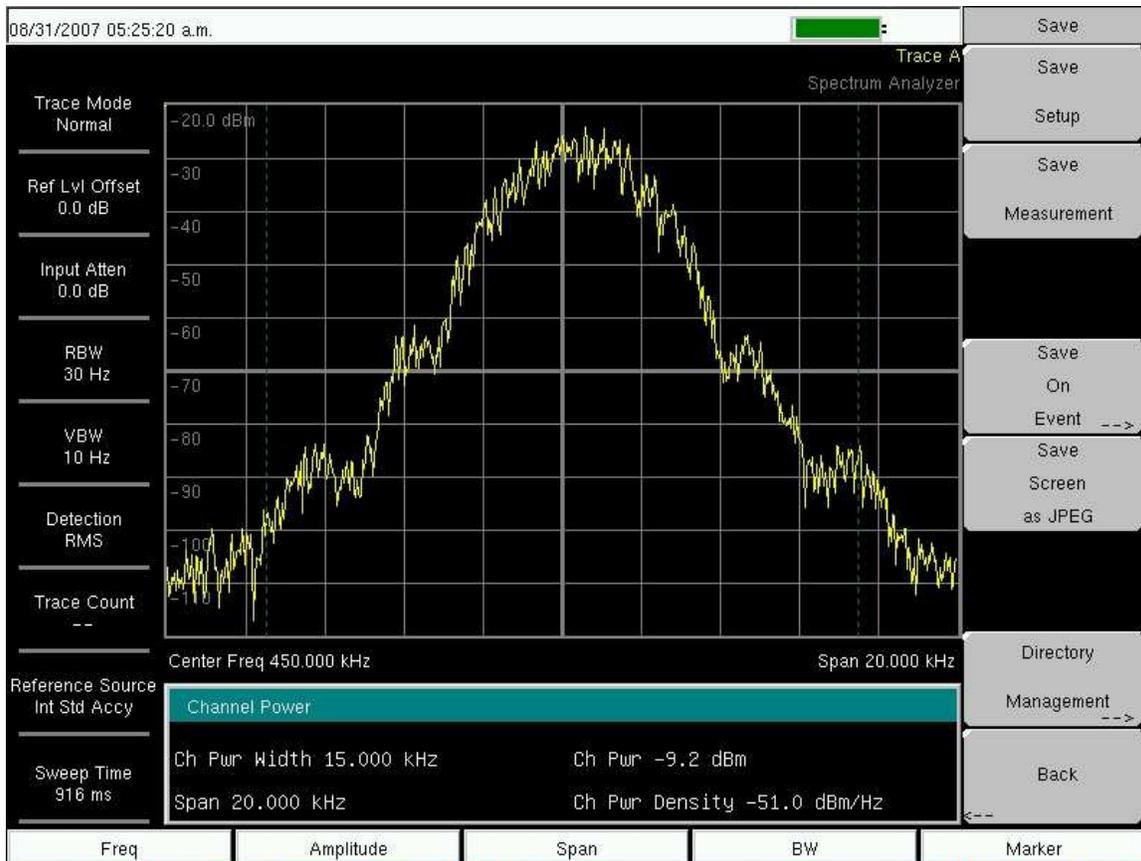
Figure 3 ID-800 450 kHz IF with a DStar Signal Prior to Detection
