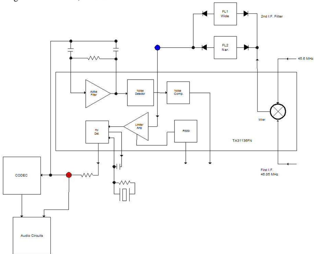
Figure 1 ID-800 IF Detector Stage
