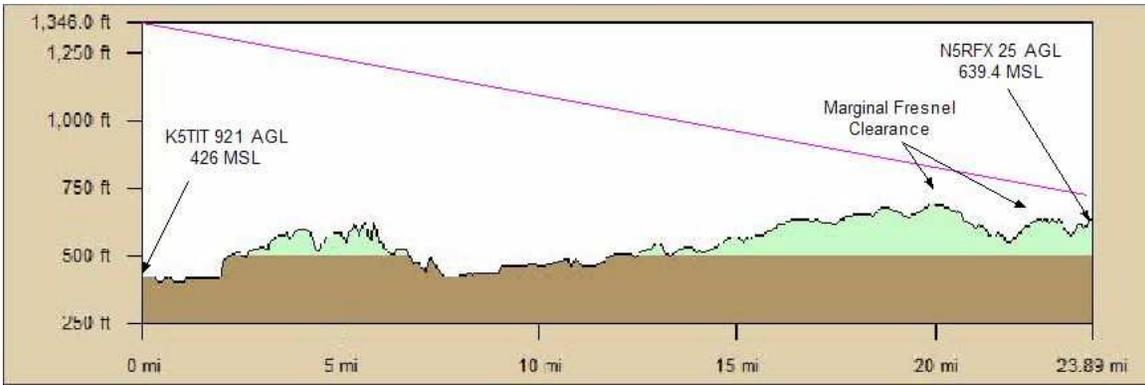
**Figure 5 K5TIT to N5RFX Terrain Profile**
